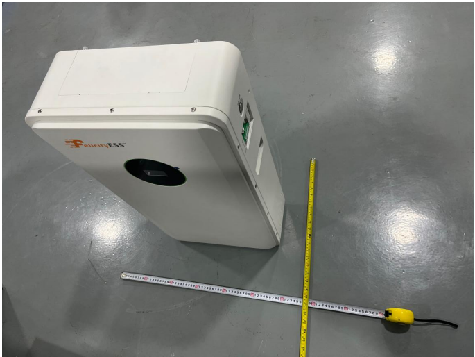
Battery (LUX-E-48100LG03, 51.2V, 100Ah, 5.12kWh)
